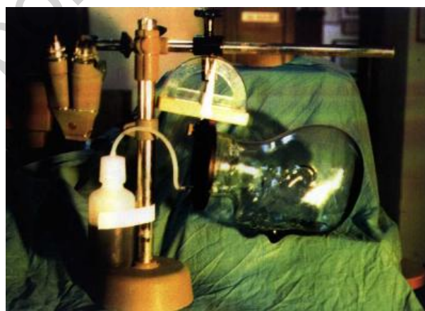
Figure 5. Specially modeled head for fluid flow simulation.
