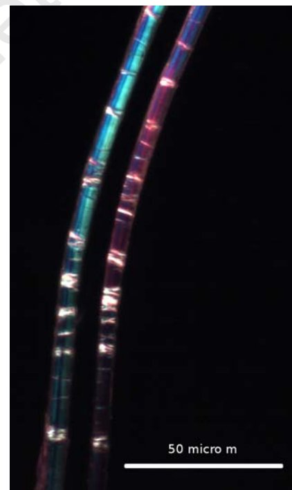
Figure 1. Polarized light microscopy image of two flax fibres from the Turin Shroud showing dislocations as white bands across the fibres.
